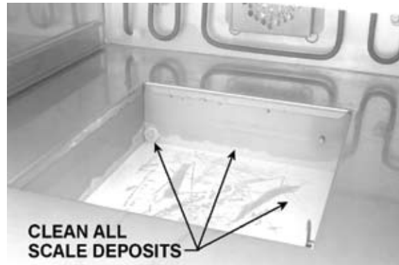
Figure 1 - Clean scale from evaporator.
