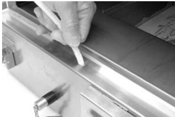
Figure 2 - Clean trough with pipe cleaner.
